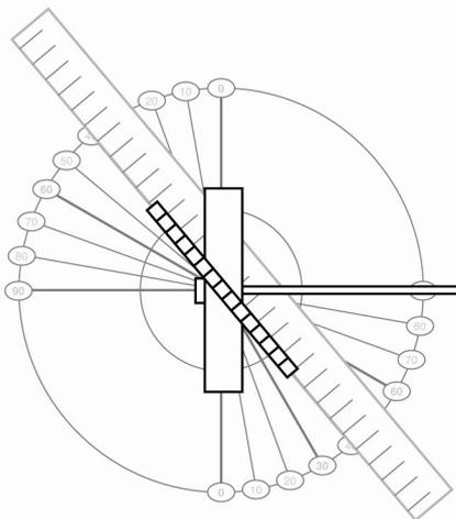
1. Hold the rotor hub over the template, and look straight down from above. Adjust its position, so that:
